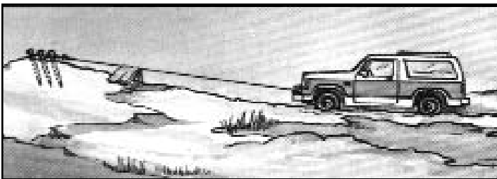
Stakes driven in solid earth and chained together make a good anchor point for self-recovery when no solid anchor point is available.
