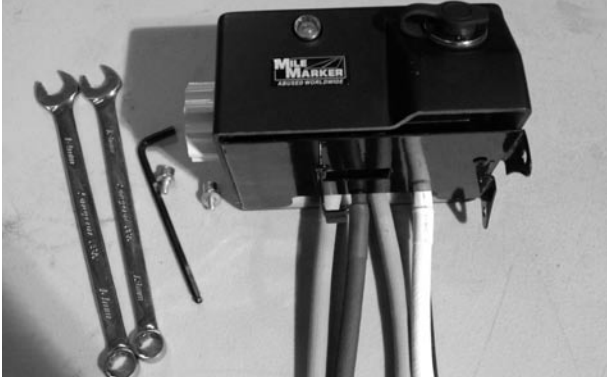
2-1: Control Box and Tools Needed: 14mm & 13mm Wrench, Metric Allen Wrench Set
