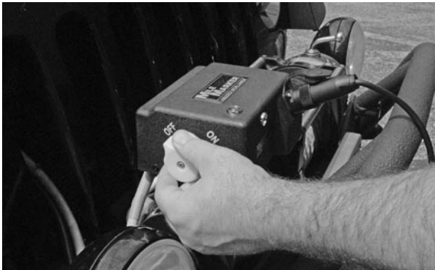
3-5: Rotate Orange Kill Switch from "OFF" position.....
