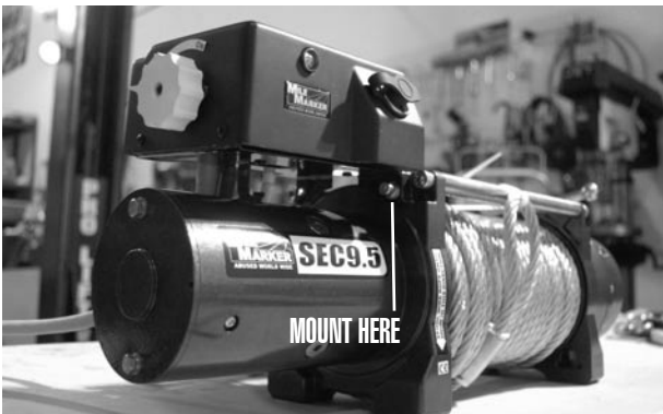
2-3: Front Control Box Mounting Point with Screw
