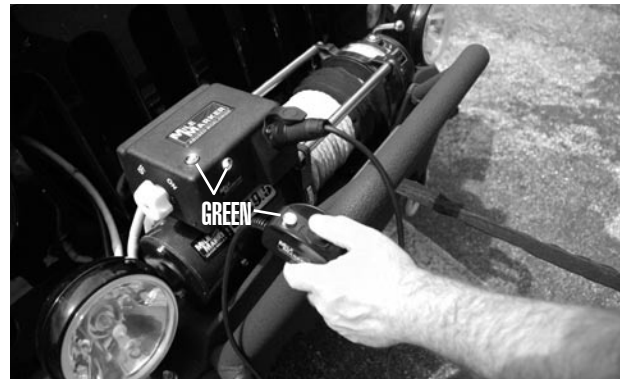
3-8: Toggle Down: Power in, "Green" LED
