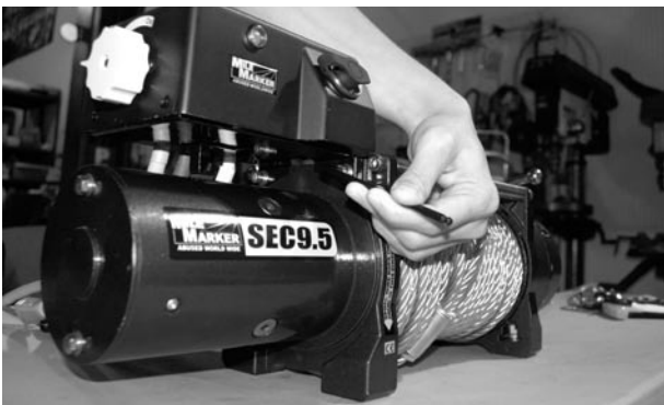
2-4: Secure Box With Allen Wrench
